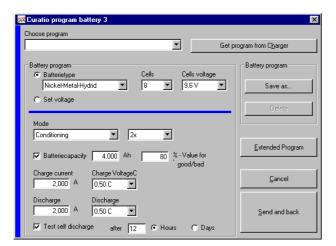
In the window "program", all parameters for discharging and charging the battery can be set and then sent to the *curatio* APL1/4.
