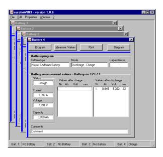
When the program "curatioWIN III" starts, the APL-4 requests the battery program and the battery measurement values from the charger that may have already been entered, and displays them. If there is no charger connected, a message to that effect is displayed. The footer in the window "program" will show the condition of the charger channels. The charging device curatio APL-1 offers one active window, the curatio APL-4 four windows.
